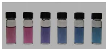
Figure 2: Suspensions of branched gold nanoparticles with a color going from red to blue.
