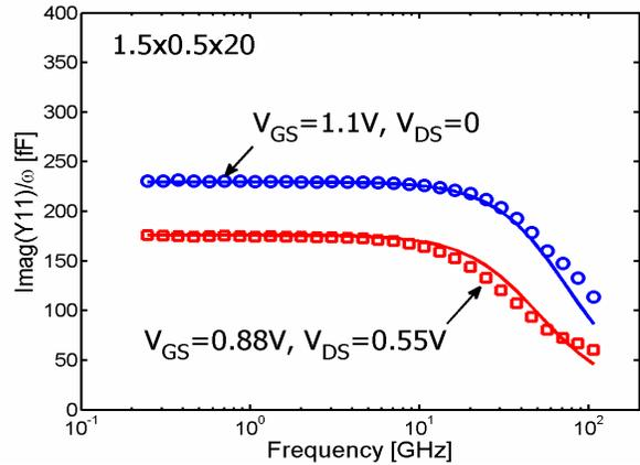
Figure 6: Measured (symbols) and simulated (solid lines) gate input capacitance,  $Imag(Y_{11})/\omega$ , vs.  $Freq.$  for a  $L=0.5\mu m$  nFET under two biases. The non-quasi-static (NQS) effect is observed and properly modeled.
