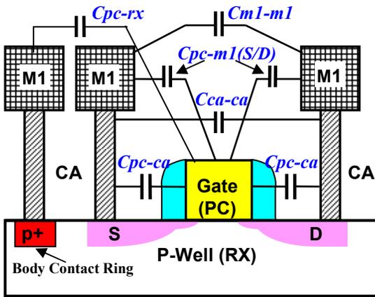
Figure 1: Wirecap network to be modeled.
