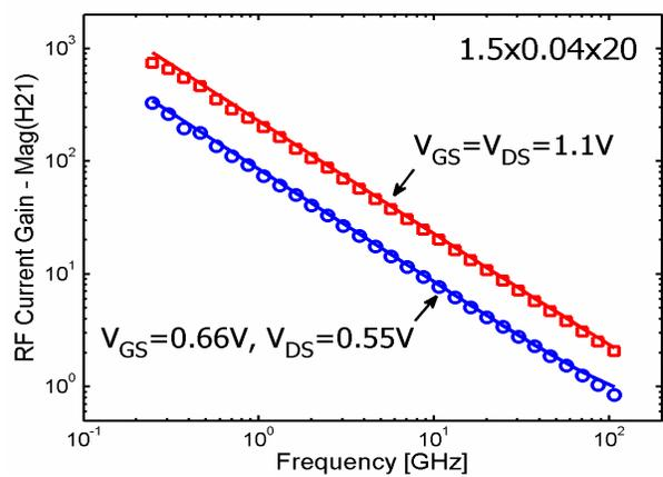
Figure 8: RF current gain,  $Mag(H_{21})$ , vs.  $Freq.$  curves for a  $1.5 \times 0.04 \times 20$  ( $W/L/nf$ ) nFET. The symbols are for hardware data and the solid lines for the model results.
