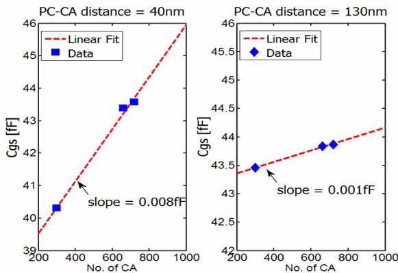
Figure 2: Measured  $C_{gs}$  vs. No. of CA curves for  $3 \times 0.04 \times 60$  ( $W/L/nf$ ) nFETs with two different PC-CA distances, 40nm (left) and 130nm (right). The  $C_{pc-ca}$  (per CA) values can be extracted from the slopes of the two dashed lines as 0.008fF and 0.001fF, respectively.
