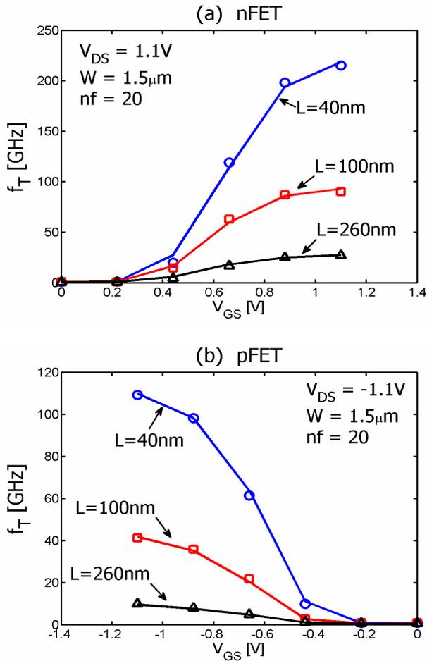
Figure 9: Cut-off frequency ( $f_T$ ) vs.  $V_{GS}$  curves for (a) nFETs and (b) pFETs, each at three different gate lengths ( $L = 40\text{nm}$ ,  $100\text{nm}$ , and  $260\text{nm}$ ).  $W=1.5\mu\text{m}$ ,  $nf=20$  and  $|V_{DS}|=1.1\text{V}$ . It is clear that the model results (solid lines) well match the measurement data (symbols) at a broad range of device geometries and voltage biases.
