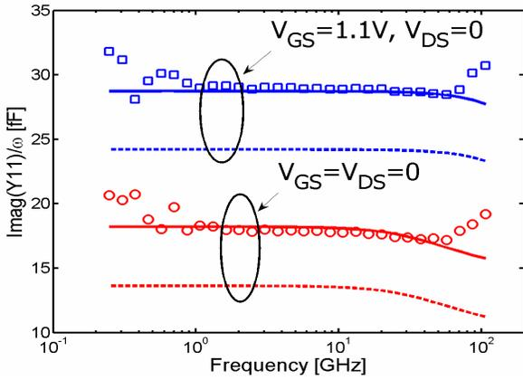
Figure 3: Gate input capacitance,  $Imag(Y_{11})/\omega$ , vs.  $Freq.$  curves for a  $1.5 \times 0.04 \times 20$  ( $W/L/nf$ ) nFET. The symbols are for hardware data, and the solid (dash) lines are for the simulation results with (without) the wirecap model enabled.
