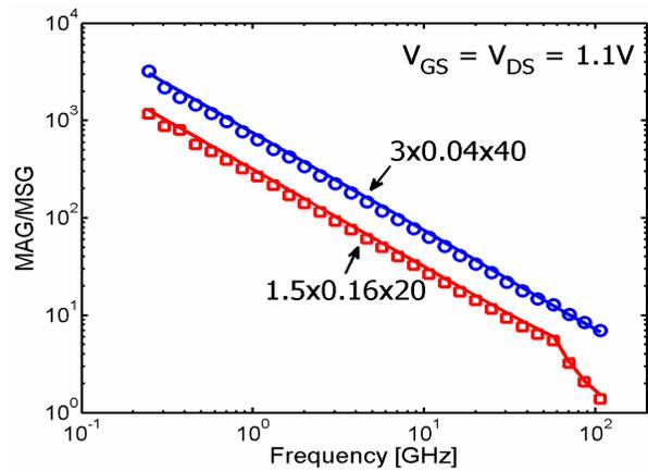
Figure 7: Maximum Available Gain (MAG) or Maximum Stable Gain (MSG) vs.  $Freq.$  for nFETs at two different sizes ( $W/L/nf$ ). The symbols are for hardware data and the solid lines for the model results.
