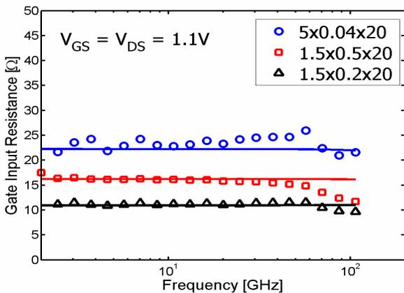
Figure 5: Measured (symbols) and simulated (solid lines) effective gate input resistance,  $Re\{(I+S11)/(I-S11)\} - 50\Omega$ , vs.  $Freq.$  for nFETs at three different geometries ( $W/L/nf$ ).
