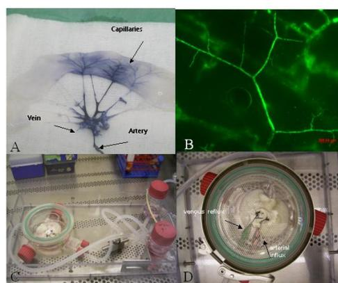
Figure 1: A) vascularized matrix with stained capillary network B) seeded capillaries of the matrix with fluorescence marked liver endothelial cells, C) Liver module with vascularized matrix and pressure sensor, D) 3D human vascularised test system with arterial and venous access
