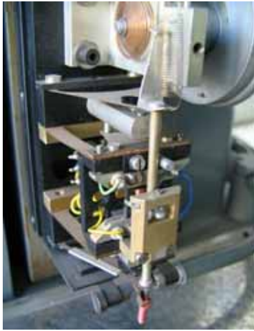
Fig. 1. The measuring stylus kit of Talystep
