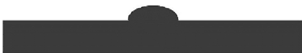
Figure. 4 Flow front shape at t=20 sec. Simulated result for no slip boundary condition without surface tension.
