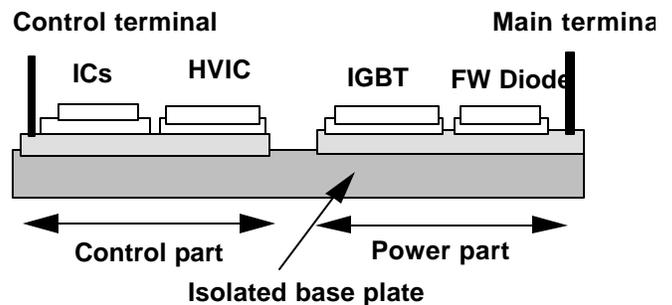
Figure 10: Schematic of ASIPM assembly.
