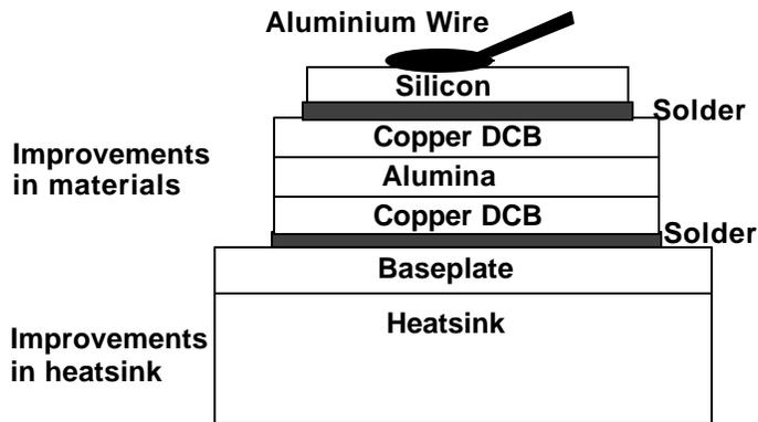
Figure 11: Schematic of conventional module assembly.
