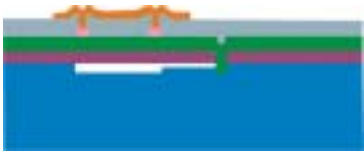
Fig.3. The cross-section of an absolute pressure sensor
