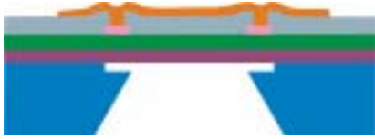
Fig.2. The cross-section of a differential pressure sensor
